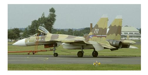
A bold, new combat aircraft designed by the legendary Sukhoi Design Bureau and now undergoing tests in Russia has taken aim at America's next-generation fighter, the F-22. The Russian challenge comes in the form of the single-seat Sukhoi S-37, the world's first combat aircraft to successfully exploit forward-swept wing (FSW) technology.
