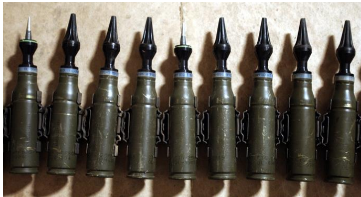
Depleted uranium is used to harden bullets and mortar shells
