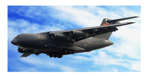
The first Xian Y-20 military transport aircraft was delivered to the People's Liberation Army Air Force (PLAAF) on June 15. Developed by Xian Aircraft Corporation, the Y-20 has an empty weight of 110 short tons, making it the largest military aircraft currently in production—larger than Russia's Ilyushin Il-76. Boeing's C-17 Globemaster III is bigger than the Y-20—the C-17's
